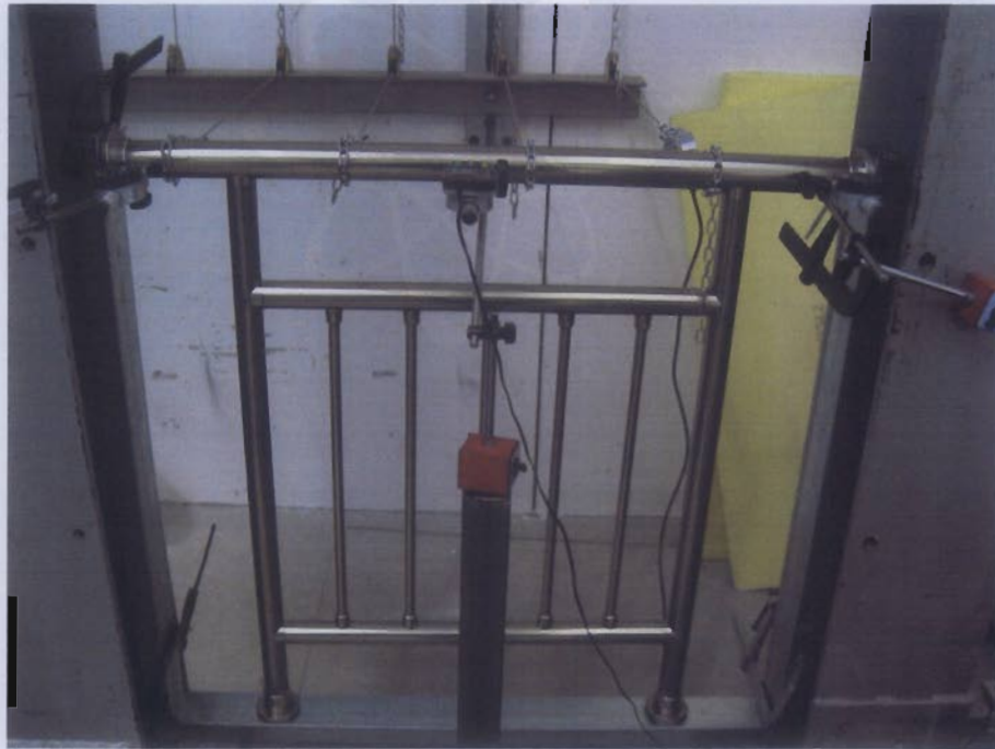
Photo of specimen subjected to uniformly-distributed horizontal loading
