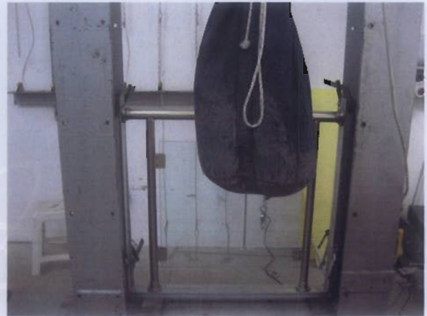
Photo of specimen after impact at handrail midpoint
