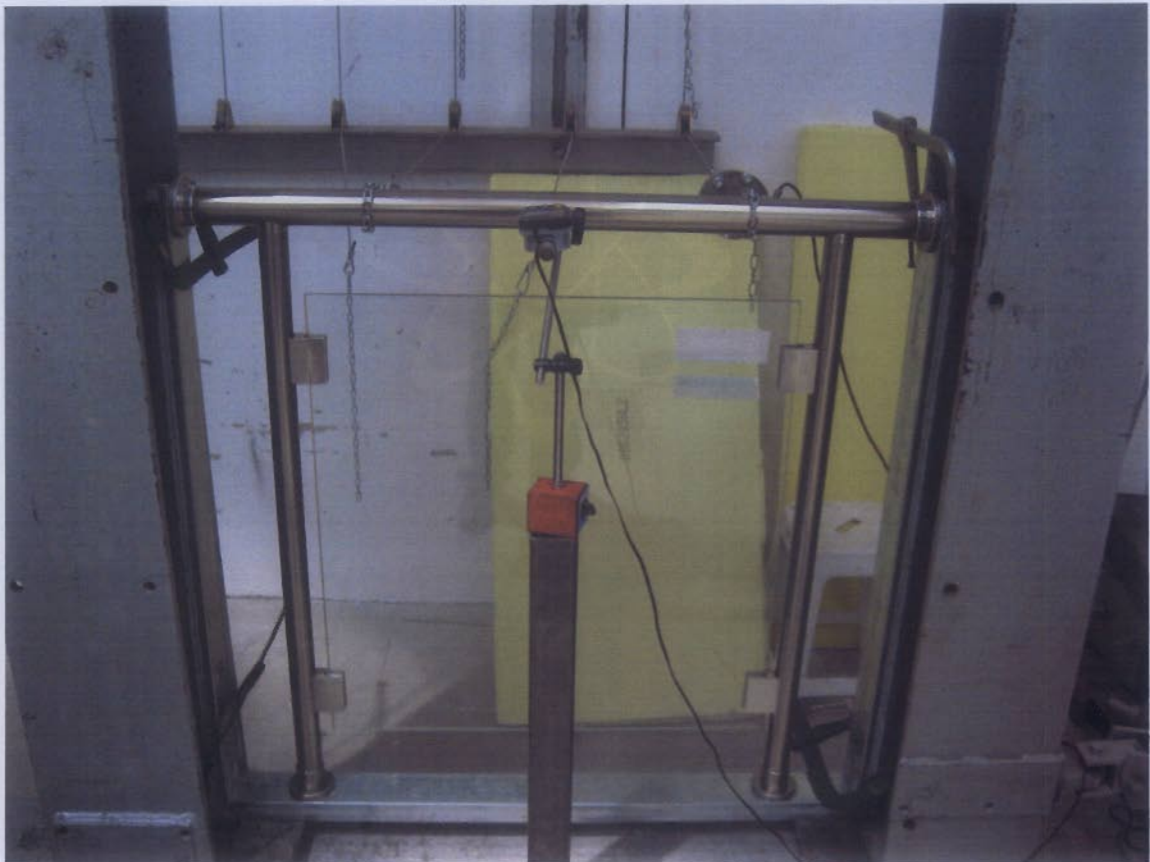
Photo of specimen subjected to horizontal static loading
