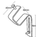
**ROOF TILE BRACKETS for PANEL 50mm**
