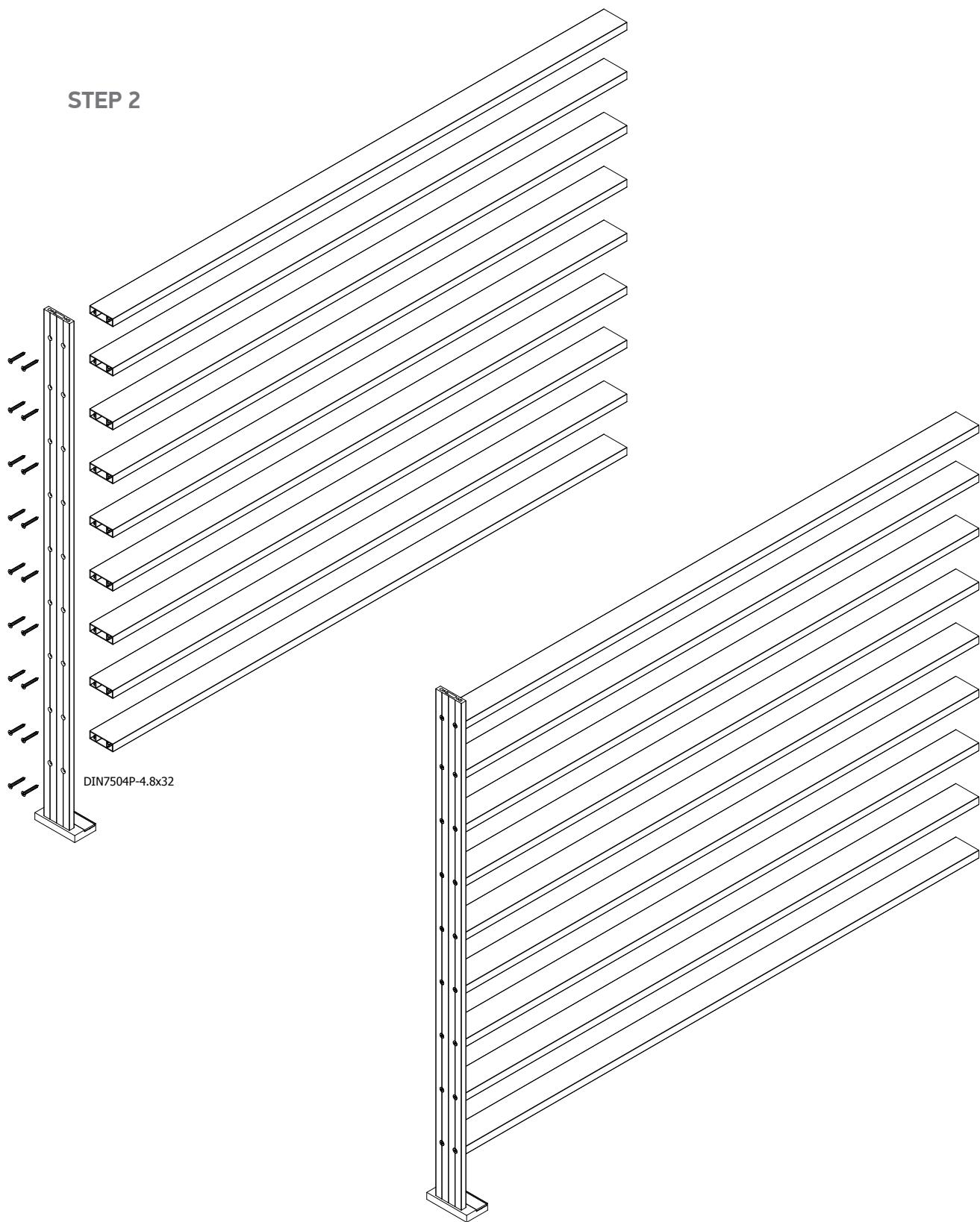
We screw the inner rails FSN-302 onto the post FSN-100.
