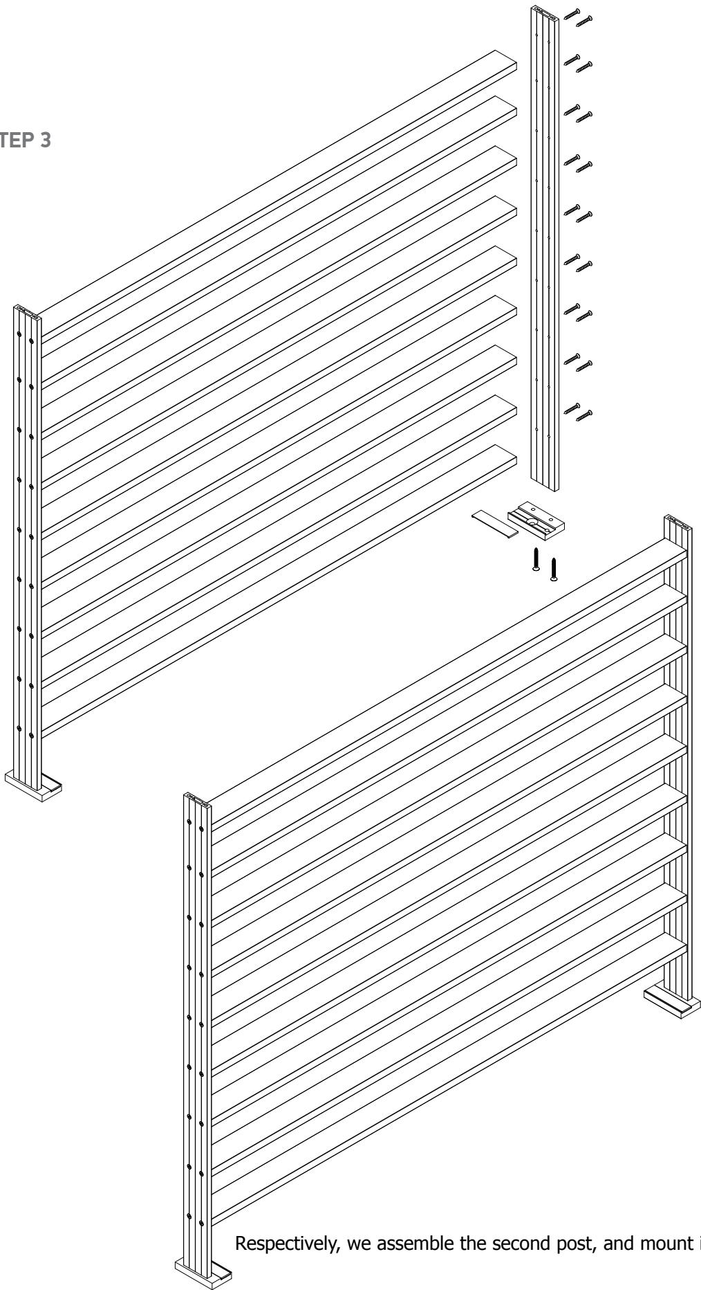
We predrill the bottom handrail part FSN-201, and then we mount it onto the awaiting rail, and we screw firmly onto the two posts, to the given positions.
